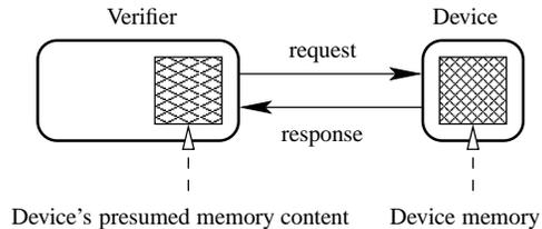
**Figure 2. Generic external memory verification.** The verifier has a copy of the device’s presumed memory, and sends a request to the embedded device. The device can prove its memory contents by returning the correct response.
