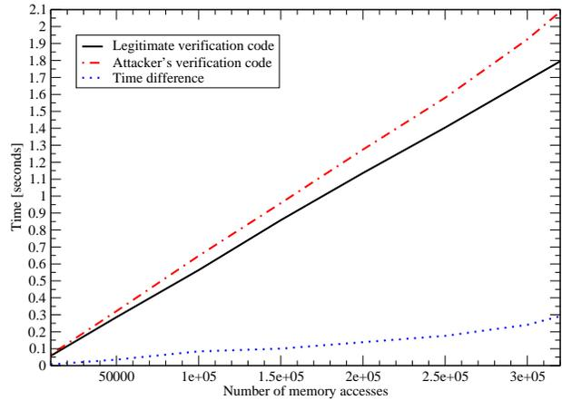
**Figure 5. Result from our implementation. Time difference of legitimate code versus attacker code. The more memory locations we include in our checksumming procedure, the larger the time difference between the legitimate and attacker.**
