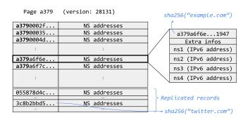
Fig. 2: Structure of a PageDNS page. The highlighted detail on the right shows the structure of a single record for the SLD example.com.
