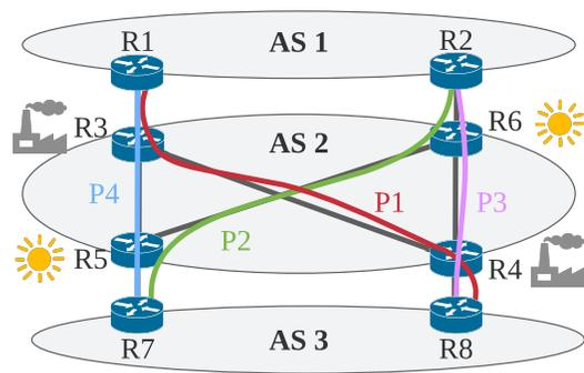
Figure 1: Inter-domain paths differ in the carbon emissions associated with data transmission, and carbon-aware path selection can leverage these differences to reduce the carbon footprint of senders.
