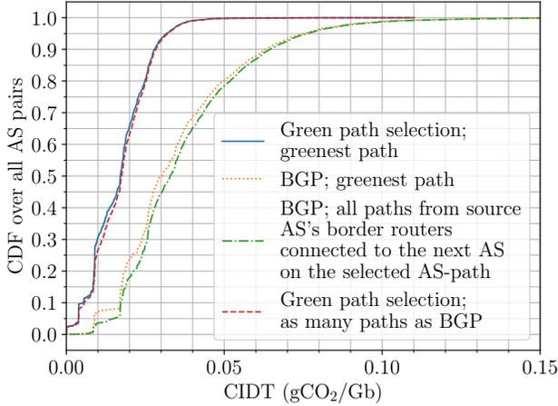
Figure 3: CDFs of CIDT for every AS pair, both for paths from green path selection and BGP.
