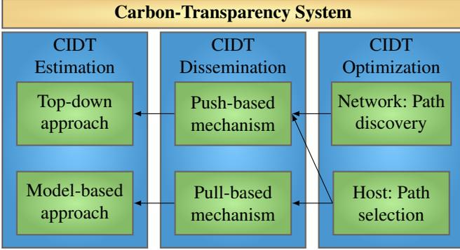
Figure 2: Overview of carbon-transparency system. An arrow from component *A* to component *B* indicates that component *A* relies on data generated/transferred by component *B*.
