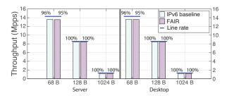
Figure 7: Switching performance of the server and the desktop for one port activated, and 68, 128, and 1024-byte packets.
