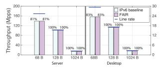
Figure 8: Switching performance of the server and the desktop for all ports activated, and 68, 128, and 1024-byte packets.
