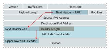
Figure 6: IPv6 packet with FAIR Extension Header.
