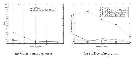
Fig. 4. Spread of Average Error for the different schemes, DOI=0.2
