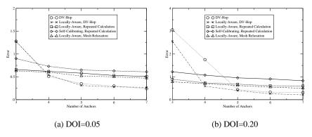
Fig. 3. Average Error with Varying Number of Anchors
