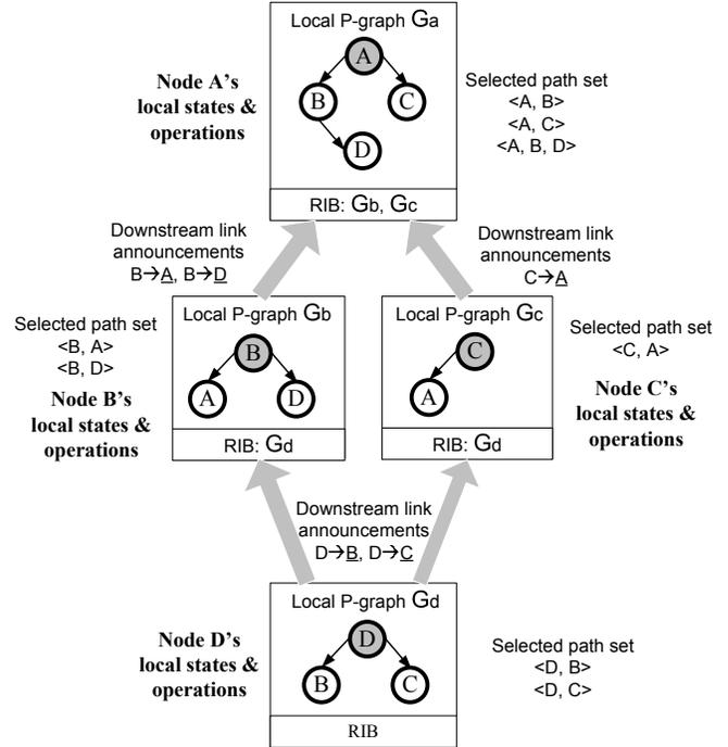
Figure 3. A simple example of Centaur operations and states. A gray node denotes the root of a P-graph. Nodes with underscores in the downstream link announcements are marked as destinations.
