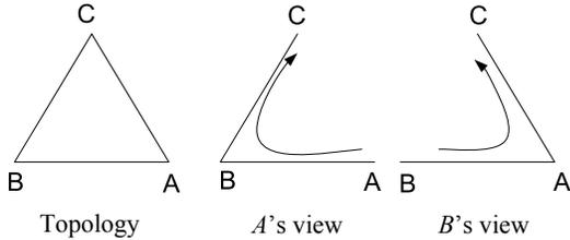
Figure 1. Loop in nodes with different topologies. Either  $A$ 's or  $B$ 's topological view contains only one path to  $C$ . To send a packet to  $C$ ,  $A$  has to use  $B$  as the next hop, while  $B$  would send the packet back to  $A$  since  $B$  is not aware of the other path to  $C$ . This example shows that even on a simple topology, it is easy to form routing loops when nodes have different topologies.
